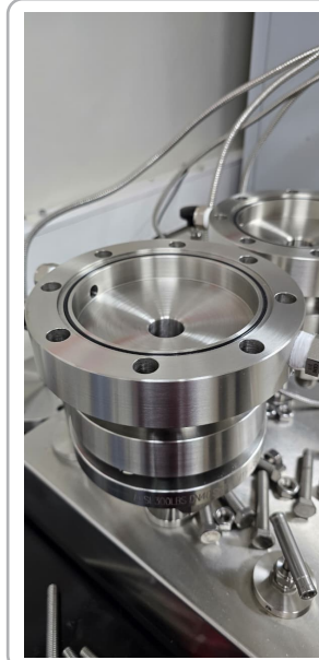
Finished custom flanged assembly
